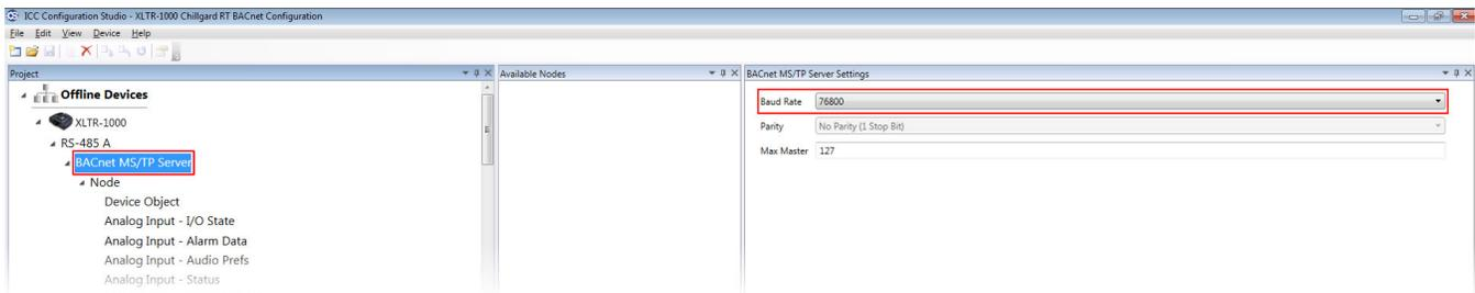
Figure 2: BACnet MS/TP Baud Rate
