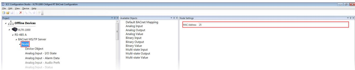
Figure 3: BACnet MS/TP MAC Address
